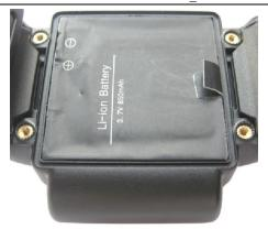
5.1.4 Close the back cover, and tighten the screws.
