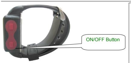
NOTE:As for ON/OFF Button,keep pressing 3 seconds is ON/OFF the tracker; while keep pressing 1 second is switch to displaying Latitude&Longitude.it displays Time,Date,Day and Battery in 30 seconds later automatically.
